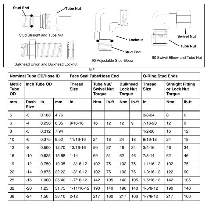
NOTE: Torque tolerance is +15%, -20%
