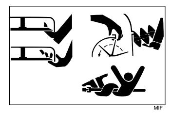
Keep hands and feet away while machine is running. Shut off power to service, lubricate or remove mower blades, augers or PTO shafts.
